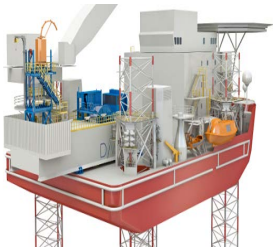
LIGHT WELL INTERVENTION CANTILEVER
